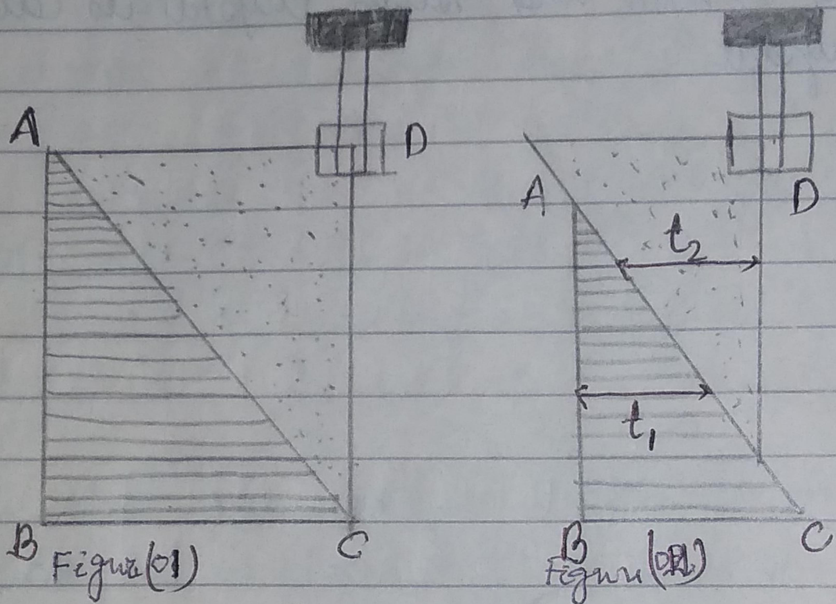
The Babinet compensator is made up of two wedge shaped quartz between section ABC and ADC having same acute angle. The wedges are placed against each other such that they form a rectangular block as shown in figure ①.
