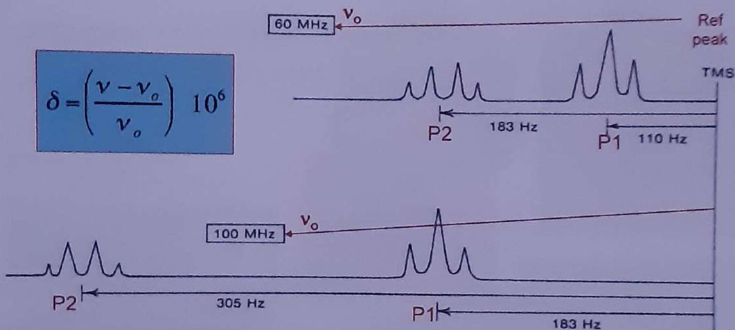
Calculate the chemical shifts of P1 and P2 using TMS as 0 ppm
