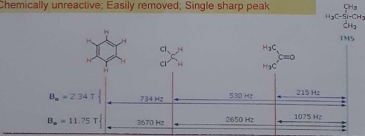
The Separation of Resonance Signals (in Hz) Increases with Increasing Field Strength
