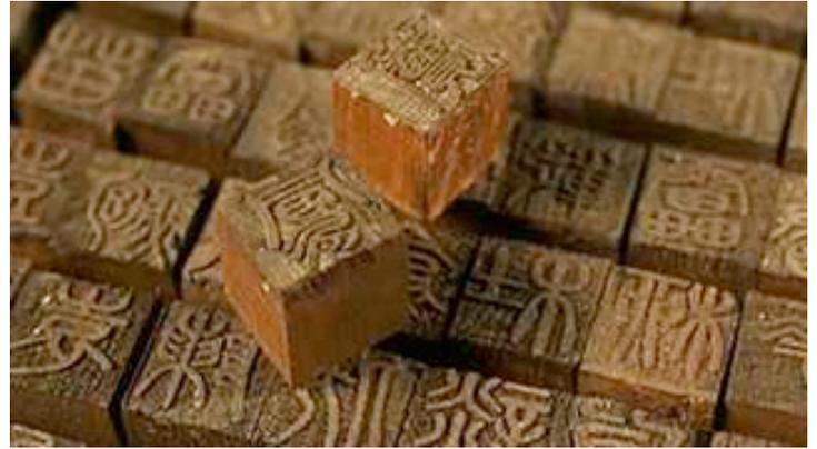
*Moveable type cut from wood. Later type was molded in clay. Thousands of characters were required for complex printing.*
